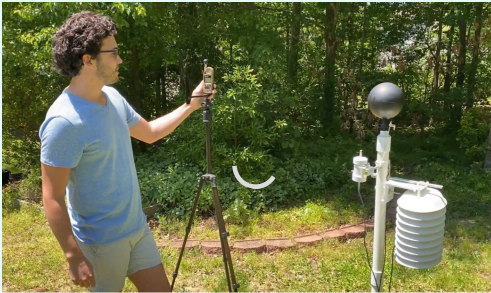
From virtual training: Jordan Clark demonstrates how to use a wet bulb globe thermometer in a video demo.
